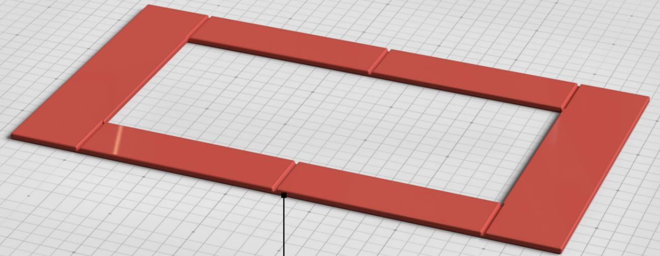
Creating this product from polystyrene would give it the rigidity it needs to break neatly along the snap lines, good dimensional stability and would be cost effective.
