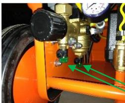
2 of the **GREEN** water valves, the last one is the water spout on the RITMO L
