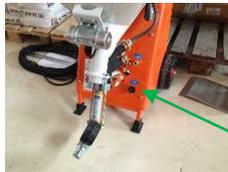
RITMO L water connector, connect water from water supply here
