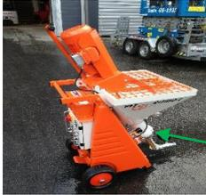
Open Water tap on the RITMO L and let all the air out of the water system. Close tap when done.
